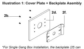
\*For Single Gang Box Installation, the backplate (2f) can be detached from the cover plate (2d) by removing the cover plate screws (2b).
